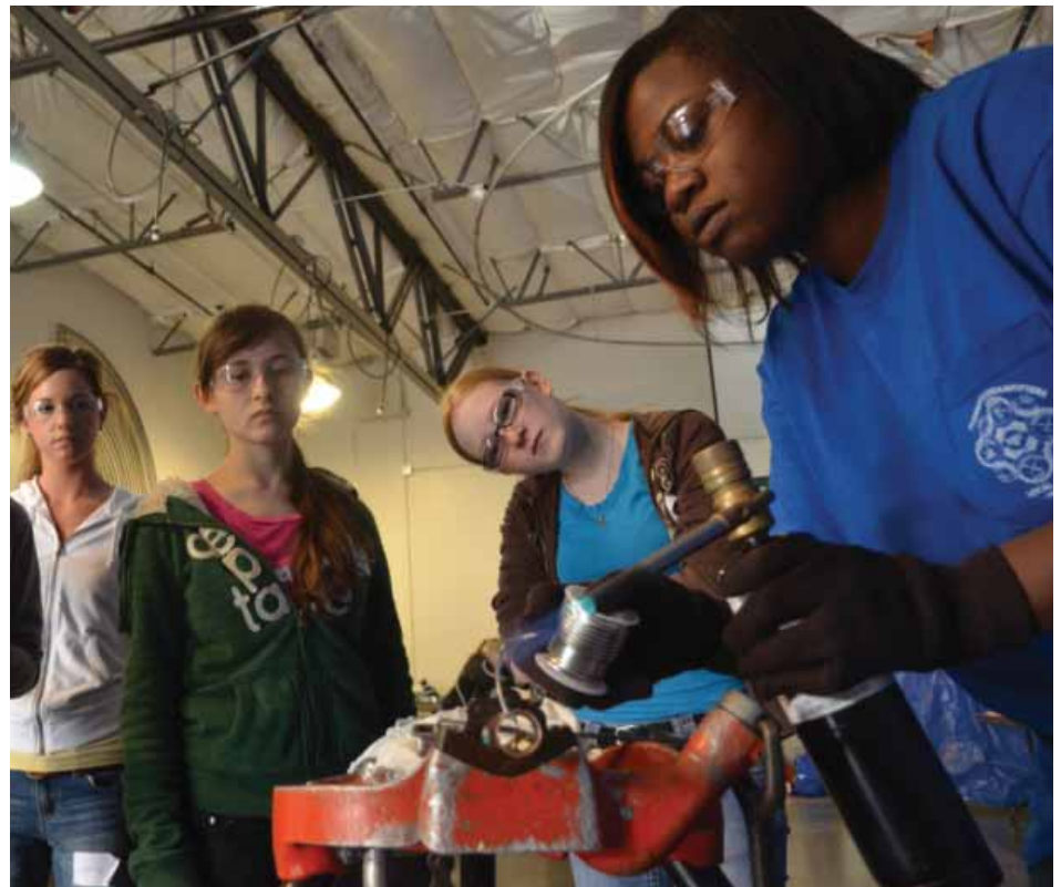
High school students learn the basics of soldering copper from Nichet Newsome (right) in a workshop with Local 290 Plumbers and Steamfitters Apprenticeship.
